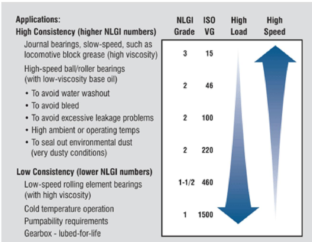
**Figure 2. Grease Consistency**
