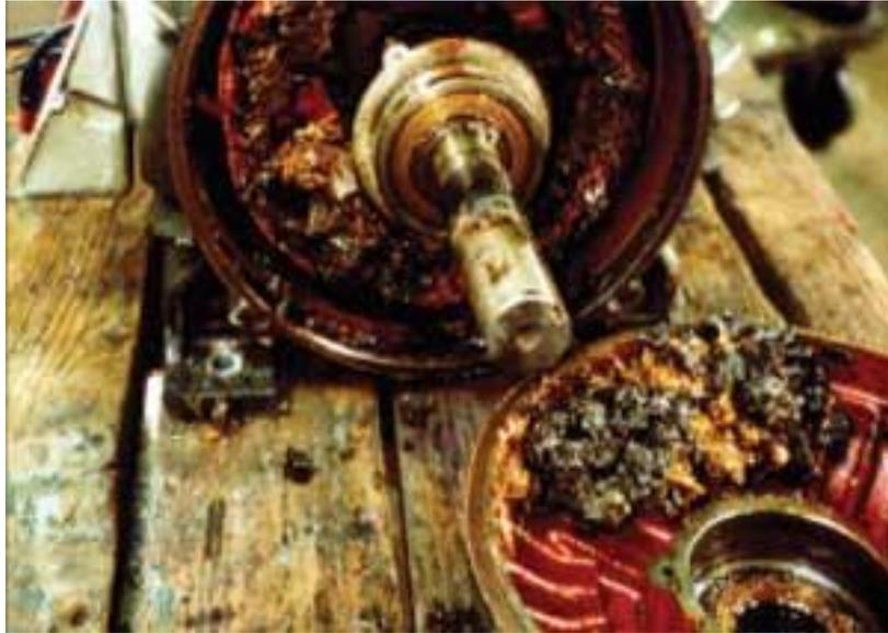
**Figure 8. Overgreasing caused inside of motor to fill with grease.**
