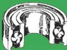
Figure 5. Sealed Bearing
