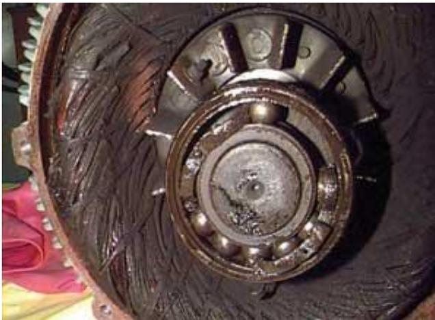
**Figure 6. Overgreasing Failure**
